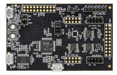
The development kit comes with necessary software including InvenSense Motion Link, a GUI based development tool and embedded Motion Drivers for IIM-42652.
