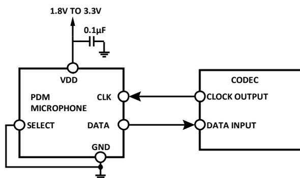
**Figure 1. Mono PDM Microphone Connection to Codec**
