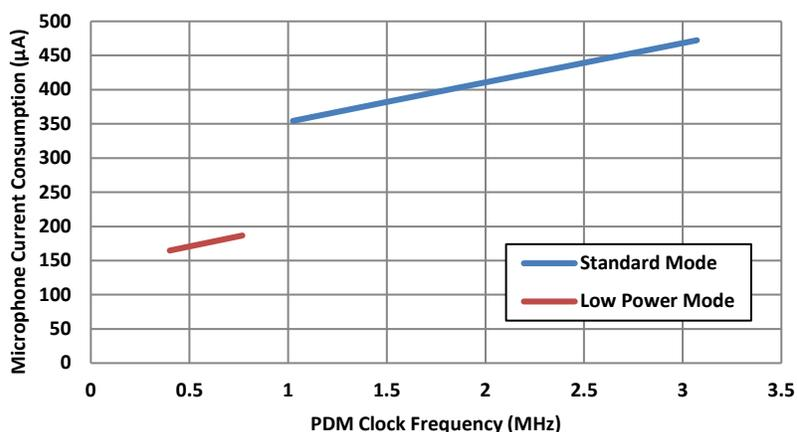
Figure 2. ICS-41350 Current Consumption at Different PDM Clock Frequencies ( $f_{PDM}$ ),  $V_{DD} = 1.8\text{ V}$
