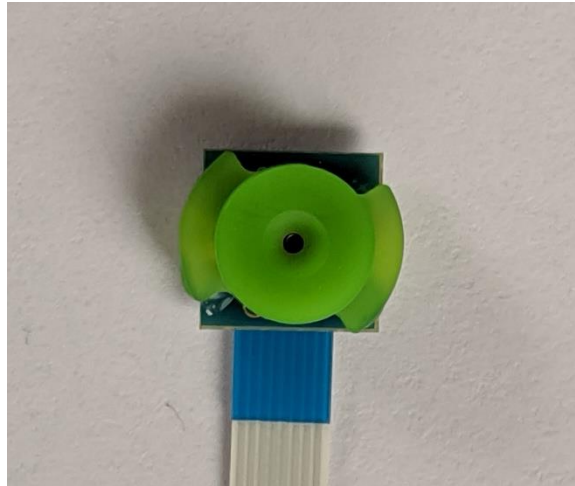
Figure 1. Chirp CHx01 module with acoustic horn
