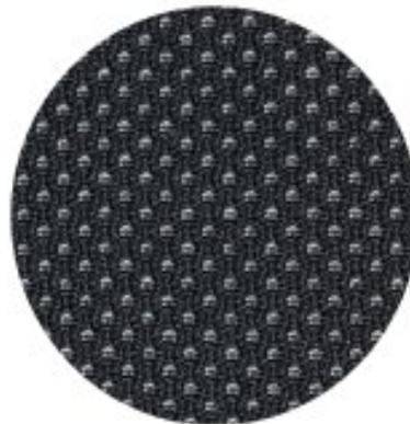
Figure 12: Acoustic mesh fabric used to cover top sound port
