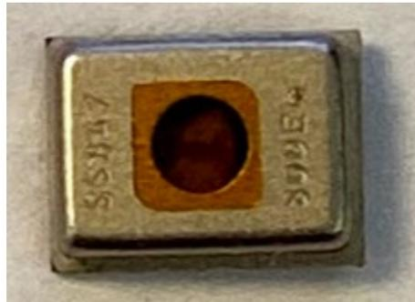
**Figure 20: Top port of ICS-40800 with tape cover**
